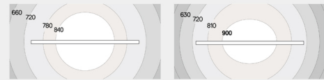
A.39 Sharp refractive emission - black louvres 1184 mm - direct only Installation h 3200 mm - Desk h 750 mm Isolines (lx) on a desk 1600x800 mm UGR < 16
